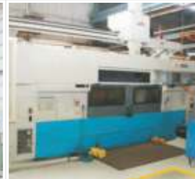
Fully automatic twin spindle, twin turret machine
