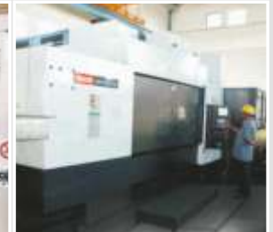
Vertical machining center with pallet hanger
