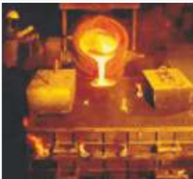
A large pump component being poured
